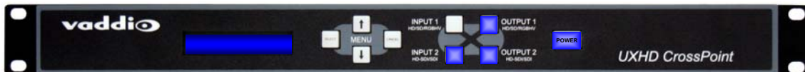
Figure 4: After this set-up, by touching the INPUT 2 button on the front panel, the UXHD will display the outputs assigned and the format of each output. By touching the OUTPUT 1 or OUTPUT 2 buttons, the backlit blue LED will turn off and the output will be toggled to black screen, allowing on the fly changes or on/off switching as needed.
