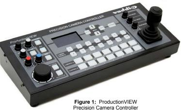
Two Precision Camera Controllers can be linked together to allow the user to control all cameras from either controller (but not concurrently, one controller at a time). The system is capable of storing up to 14 pan, tilt and zoom position presets per camera. Two discrete control buses can be configured to select PTZ cameras, as well as control an external switcher or mixer via either RS-232 or tally outputs on the back of the console.
