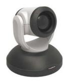
The camera optics shall feature a 12x optical zoom lens with seamless transition to 1.67x digital zoom, for a total zoom range of 20x. The camera shall use a 1/2.3-type, high-speed, low noise, back-illuminated CMOS sensor with 9.03 total megapixels, producing native 2160p/30 (3840 x 2160) video images without scaling.
