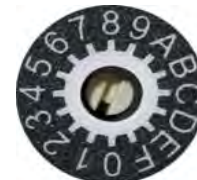
Point the notch in the switch stem to assign the rotary position
