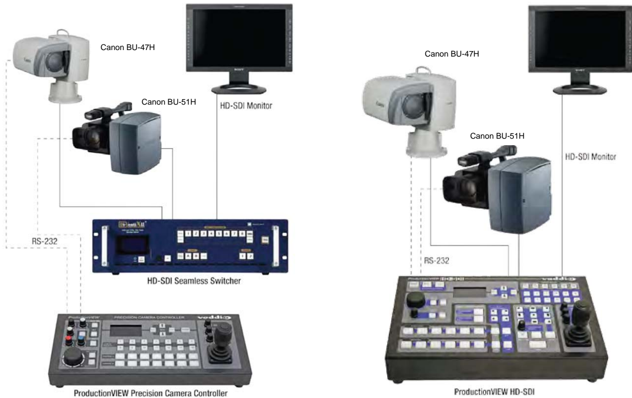
Figure 2: Basic connectivity of the BU-Series cameras with Precision Camera Controller and 3 rd Party Switcher (left) and with ProductionVIEW HD-SDI (right).
