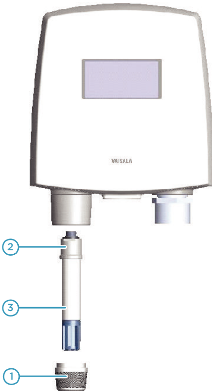
Figure 13 Removing the Humidity Probe (Fixed Probe Model)
