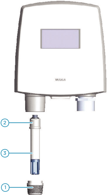
Figure 13 Removing the Humidity Probe (Fixed Probe Model)
