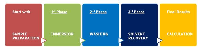
First, the extraction is made by immersion of the sample in the boiling solvent. This step is followed by a rinsing phase with hot solvent. Then, all the solvent evaporates and it is recovered in a condenser. The calculation of the total fat content follows gravimetrically after drying the extract.
