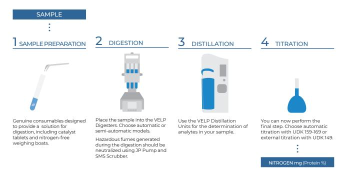
The Kjeldahl method consists in a procedure of catalytically supported mineralization of organic material in a boiling mixture of sulfuric acid and sulfate salt at digestion temperatures higher than 400 °C. During the process the organically bonded nitrogen is converted into ammonium sulfate. Alkalizing the digested solution liberates ammonia which is quantitatively steam distilled and determined by titration.
