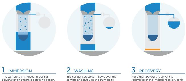
sample and through the thimble to complete the extraction process.
