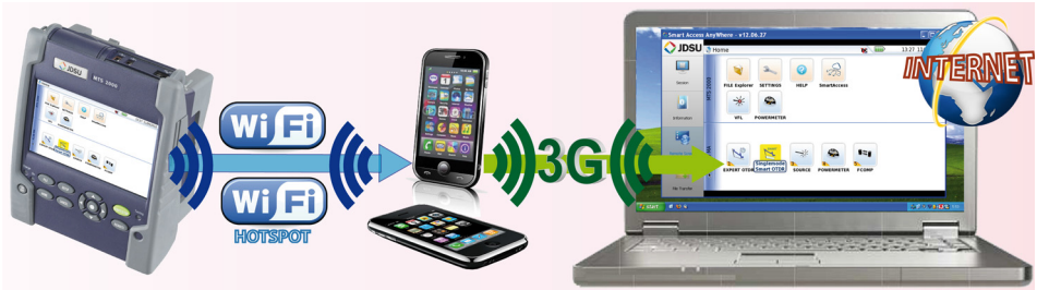
Figure 58 WiFi connection through 3G Smartphone
