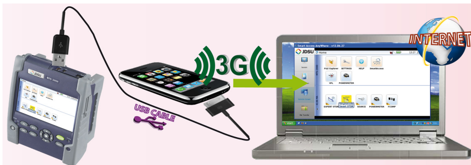
Figure 57 USB connection through 3G Smartphone
