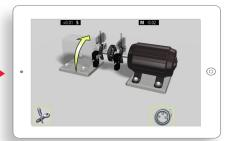
Rotate the sensors to the 12:00 position. Press the measurement icon again to take the second measurement.
