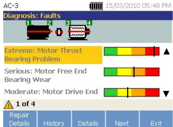
Figure 4. Automated vibration analysis can report on machine health in terms that are understandable and actionable by technicians without vibration analysis experience.
