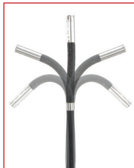
The articulating probe's ±150° viewing angle enhances inspection flexibility
