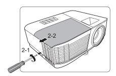
3. Remove the lamp cover and mylar from the projector.
