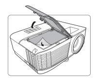
11. Tighten the screws that secure the lamp cover.
