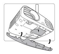
11. Tighten the screws that secure the lamp cover.
