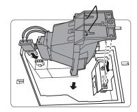
9. Insert the lamp connector and tighten the screw that secures the lamp.
