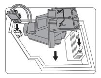
9. Insert the lamp connector and tighten the screw that secures the lamp.
