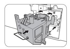
7. Tighten the screws that secures the lamp.
