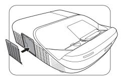
9. Tighten the screws that secure the lamp cover.
