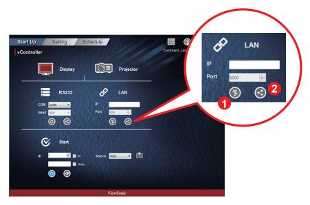
• Enter the IP address of the monitor in the IP address field. When the network settings interface is opened, press the button to PING the IP address of the monitor to see if the connection is successful.
