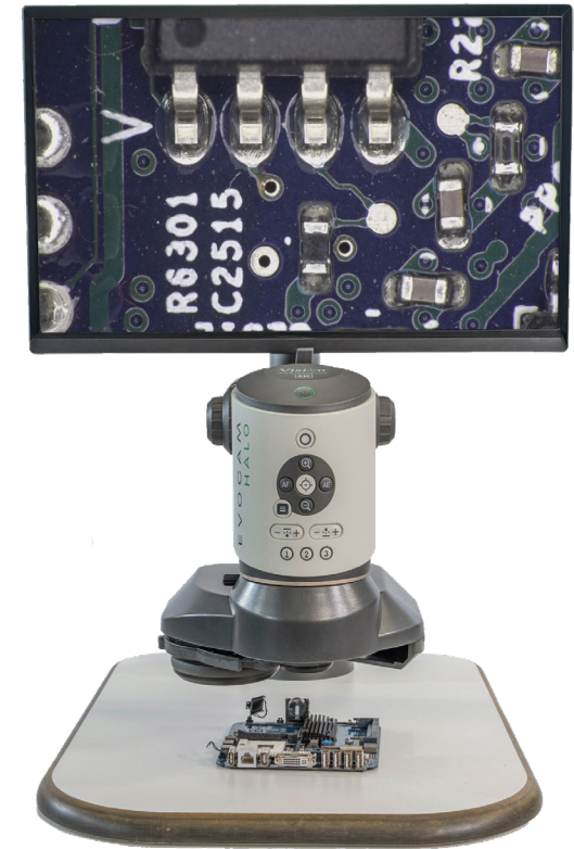
EVO Cam HALO fitted with 360-degree Oblique and Direct Viewer (ODV)
