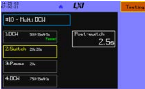
Figure 8-12 Running Switch Control Steps
