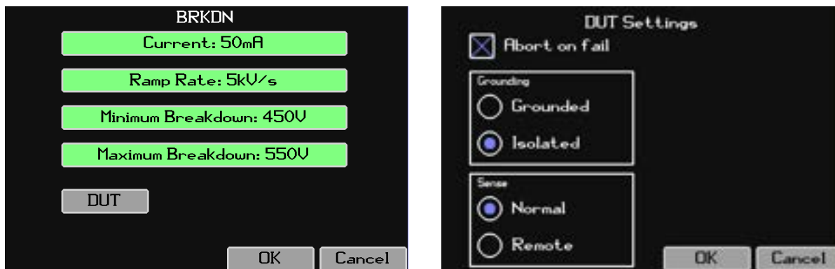
Figure 7-25 BRKDN Step Configuration Screens
