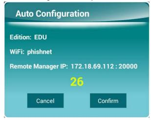
2. After the new settings take effect, the NovoConnect device will automatically report its existence to the Remote Manager. You can click on "Device Discovery" and then "Discover Devices" to bring up a discovery dialog window where you will be able to view live NovoConnect devices and add them to the device list of the Remote Manager.
