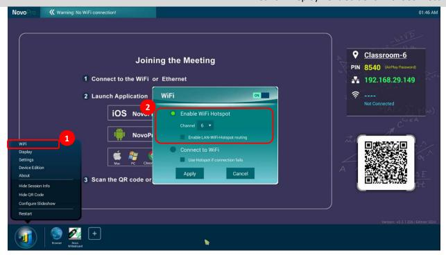
In addition, you can rename the Wi-Fi Hotspot SSID and change its security settings (security protocol and its password.) To do so, click on <u>Settings</u>  $\rightarrow$  <u>General Settings</u>  $\rightarrow$  <u>More</u>  $\rightarrow$  <u>Tethering</u> & <u>portable hotspot</u>. Then the following "Set up Wi-Fi hotspot" window pops up to allow you to make the necessary changes.
