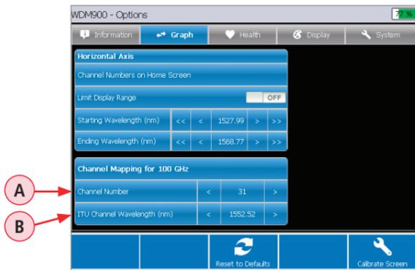
In DWDM systems using 50 GHz channel spacing, channels can be labeled using whole numbers only, using fractional numbers (such as C20 and C20.5), or using C/H notation (such as C20 and H20).
