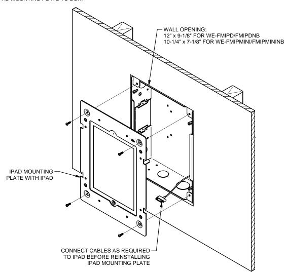
7. REINSTALL FRONT PANEL TO IPAD MOUNTING PLATE.
