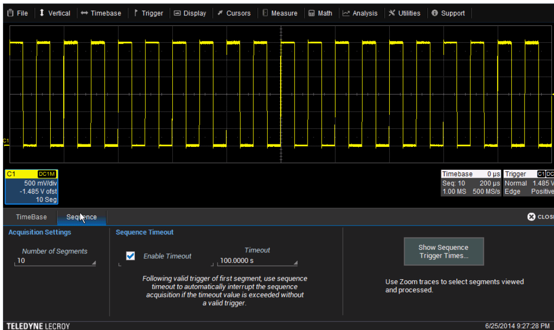
Figure 2: Upon invoking the Sequence Mode option in the Timebase tab, users are presented with the controls dialog at the bottom of the screen.
