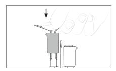
Push the grip with the fitters onto the tweezers.
