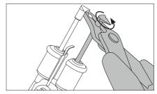
Align cartridges with JBC pliers.
