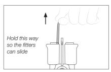
To remove the fitters, hold the grip and pull them out. Use pliers if necessary.
