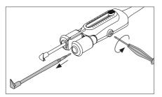
Loosen the screws and remove the cartridges.
