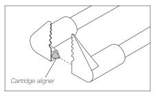
Align the cartridges in working position using a flat pliers (JBC Pliers PLR195). The conical cartridge aligner helps centering
