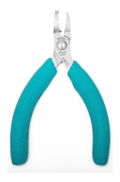
The Weller Erem Series 500 Micro is a full range of medium sized, robust, precision cutters with a wide range of head shapes. The cutters are manufactured from high grade tool steel. The cutting edges are hardened to Rockwell 63-65 HRC. The precision cutters have a nonreflecting surface, are ESD safe and resharpenable.
