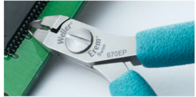
Tip cutters to remove fine pitch SMD ICs
