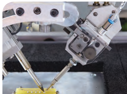
"On point" solder feeder next to the iron smoothly pulls the solder wire through the tube
