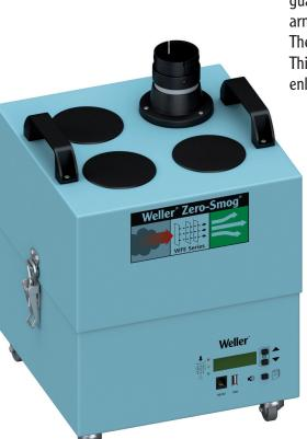
New optimized pressure control. This feature guarantees a constant air flow at every extraction arm, no matter how many arms are connected. The blower speed is adjusted automatically. This saves energy, reduces the noise level and enlarges the filter life time.
