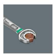
The Joker's clever double-hex geometry delivers a very positive connection with nuts or bolts - it's a perfect fit. And the exchangeable, hardened metal gripping plate in the Joker's mouth literally bites itself into the bolt, with its extremely hard tips. Both features combine to prevent slipping, even at higher torque.
