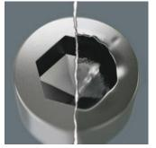
Hexagon screws can endure a problem because the contact surfaces delivering the power from the conventional tool, transferred to the screw via very small surface areas. The consequence: the screw can become damaged (rounding out). Hex-Plus tools have a greater contact surface that prevents this from happening! At the same time, as much as 20 % more torque can be applied. Good to know: Hex-Plus tools fit into every standard hexagon socket screw!
