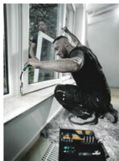
Around the corner screwdriving with the 393 S screwdriver. The flexible shaft allows to reach fixing screws in unfavourable positions. The ideal tool for screwdriving situations that are difficult to reach.
