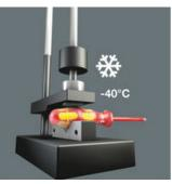
Impact strength tested at -40°C, guaranteeing safety even under extreme conditions.
