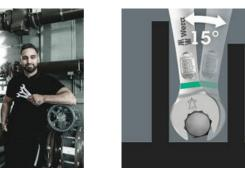
The Joker 6003 ring spanner with its special mouth geometry mouth side pivoted by 7.5° and the double hexagon profile doubles the placement possibilities when repeatedly turning the wrench 180° around the longitudinal axis. Bolts and screw heads can be "accessed" every 15°. The Joker 6003 will automatically find the respective placement point after every turn.
