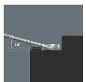
The ring side is cranked at 15° to the tool axis to prevent injury.
