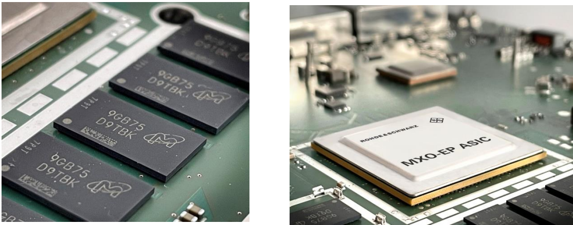
Figure 1. For R&S®MXO 4 Series oscilloscopes, the R&S®MXO-EP (Extreme Performance) ASIC contains an integrated memory controller that reads and writes to fast DDR memory. The 28 nm CMOS ASIC powering the industry's fastest deep memory update rate, has over 36M transistors and can process at 200 Gb/s.
