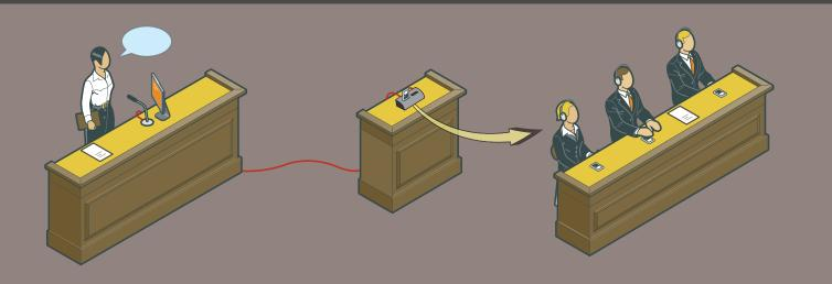
**Example 2.** You can also use the Digi-Wave Dock to deliver audio created within a Digi-Wave system to listeners of a separate sound system. Place a DLT 100 2.0 transceiver or DLR 60 2.0 receiver into the Dock. When the output is connected to a sound system or powered speaker, the Dock allows the transceiver/receiver to function like a base station receiver that connects a portable system to a fixed system.
