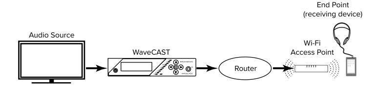
Audio is taken from the source (TV's, cable, satellite, live sound systems, etc.) and brought into the WaveCAST Server via analog or Dante connections. The WaveCAST encodes and broadcasts the audio over the IP network.
