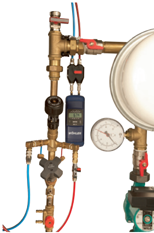
Fig. 3.1.3: Before switching on the Wöhler DC 17, with valve in the test hose adapter set to „P = 0“. The valve of the red test line remains closed.
