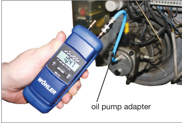
Fig. 3.3.1: Connecting the DC 17 to an oil pump
