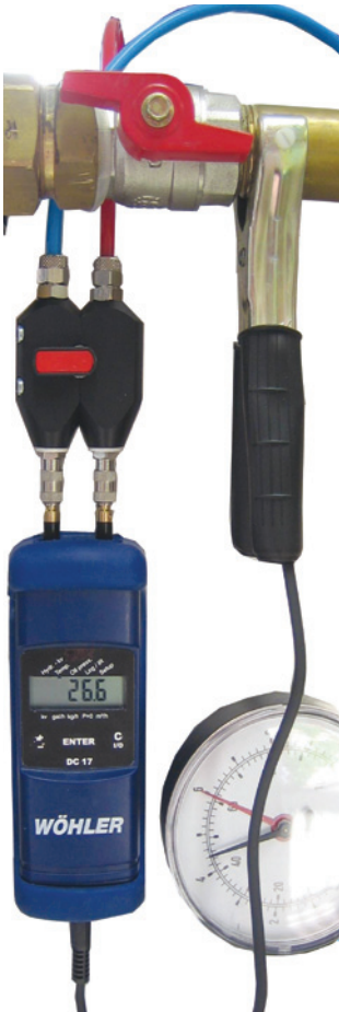
Fig. 3.2.1: Measurement of the flow temperature using temperature measuring pliers (Cat. No.: 3619)
