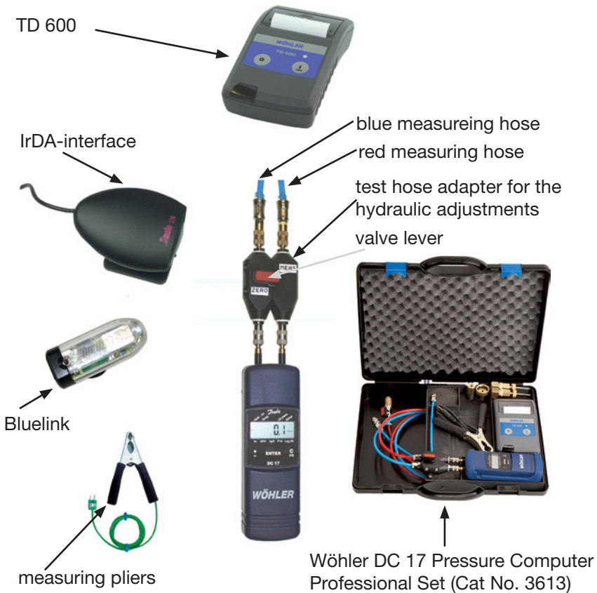
Fig. 2.2: Connections and connections of the DC 17 pressure computer for hydraulic adjustments and measuring the oil throughput
