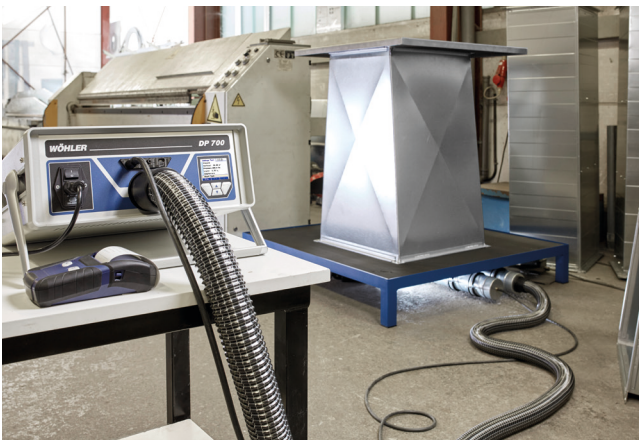
Quality control during series production of ducts and components.
