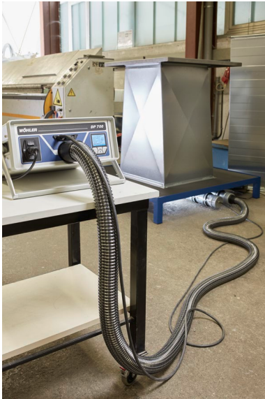
Fig. 12: Example: Measurement according to DIN EN 15727
