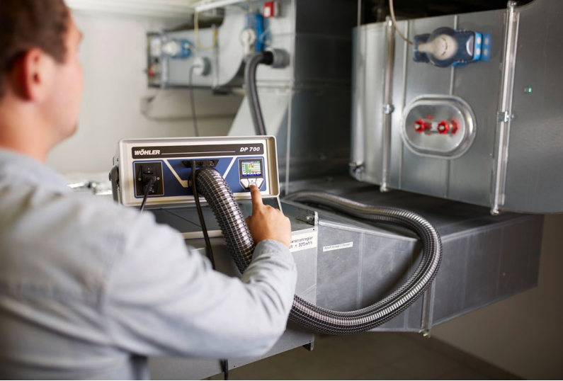
Fig. 11: Example: positive pressure measurement without adapter
