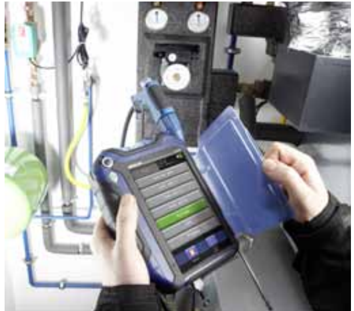
The Wohler A 550 Combustion Analyzer with protective hinged lid.
