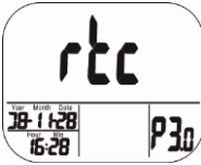
Fig. 13: Setting clock and calendar (rtc: real time clock)
