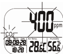
Fig. 21: Display during the CO 2 calibration
