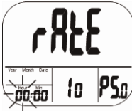
Fig. 19: Setting the sampling rate (hours)
