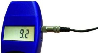
Fig. 10: Connecting the cable to the Wöhler HBF 420
