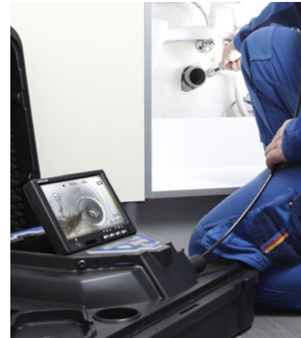
The robust color camera head is waterproof to IP 68 rating. With a diameter of just 1" it easily negotiates bends in pipes of 1.5" and larger.
