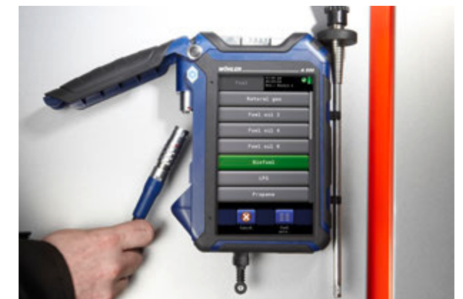
Analysis, temperature and draft - 3 functions in a single hose: Simply plug them together and fold down the protective lid.
