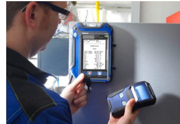
Printing out the results on the spot with the Wohler TD 100 Thermal Fast Printer.
