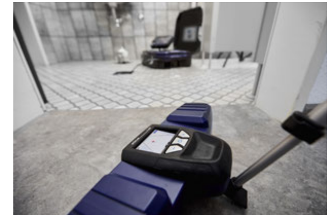
Precise location of the camera head with the Wohler L 200 Locator.
