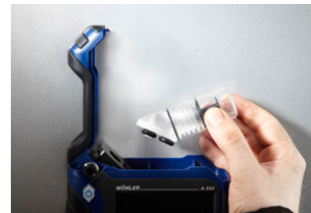
The bright blue condensate trap is able to be serviced quickly and easily.
