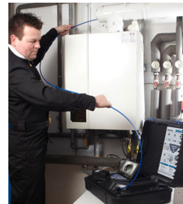
The 360° pan and 180° tiltable color camera head easily negotiates 87° bends.
