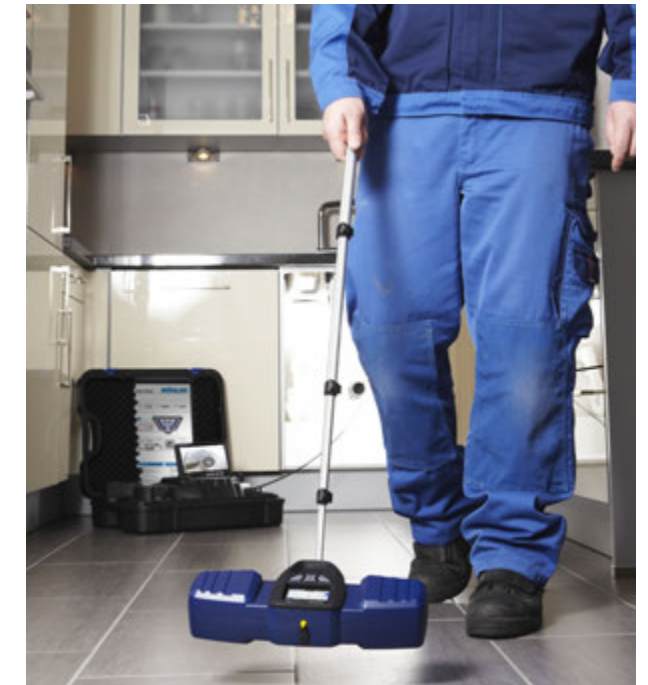
The actual distance count and the position of the head are displayed in the monitor. The Wohler L 200 Locator makes it possible to locate the camera head.
