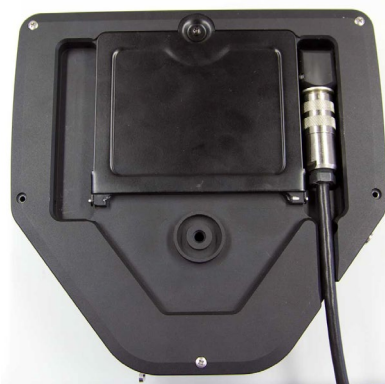
Fig. 9: Camera cable fed through guide
