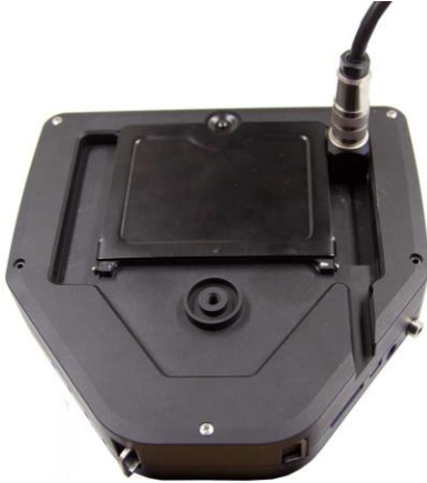
Fig. 8: Camera cable connection
