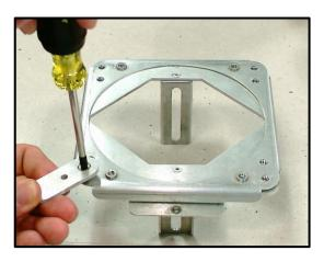
4) Slide circular plate into mounting assembly.
