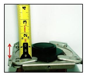
9) Adjust the camera until the distance from the front of the Mounting Tab to the end of the camera matches the ceiling thickness. Then secure camera with knurled screws.
