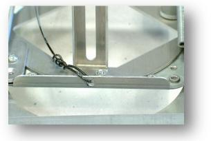
16) Loosen knurled screws and lower camera until flush with bottom of ceiling tile. A straight edge may be used to verify.
