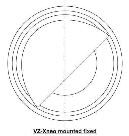
Turn swivel **top** plate counter-clock-wise to the end position. Place the cut-out of the template onto the swivel top plate.
