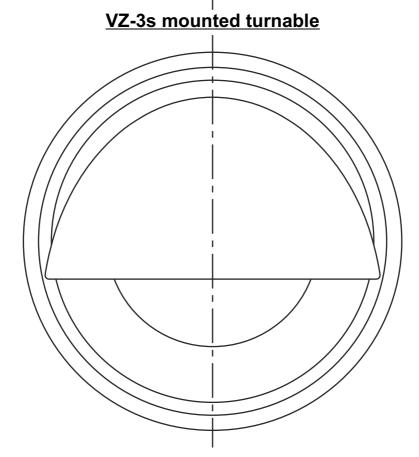
Turn swivel **top** plate to the end position in the opposite direction of desired closing down. Place the cut-out of the template onto the swivel top plate.
