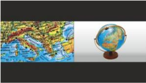
The Picture in Picture Mode offers the possibility to show two different pictures at the same time on one screen. Just press the PiP key (*assigned PRESET key*) to activate the Picture in Picture mode. The current picture (e.g. external signal, image memory) will be shown in the lower left corner and the live image will be shown in the upper right corner. The size of the live image is much bigger.
