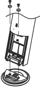
Connect all desired cables and fix them with the cable tie.
